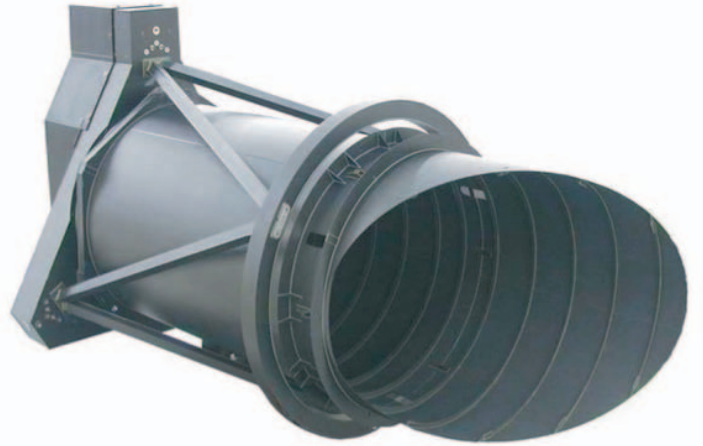
The HiRISE Camera on Mars Reconnaissance Orbiter
