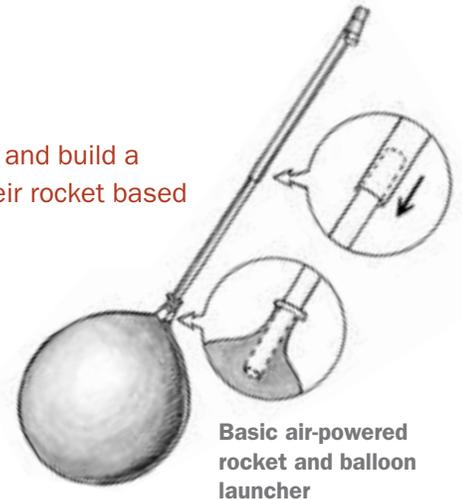
Basic air-powered rocket and balloon launcher
