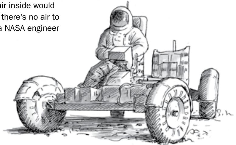
Despite these challenges, engineers designed a tire that worked perfectly when it was used on the moon. It's made of thin bands of springy metal. That helps it be lightweight, have good traction, and work at any temperature the moon can throw
