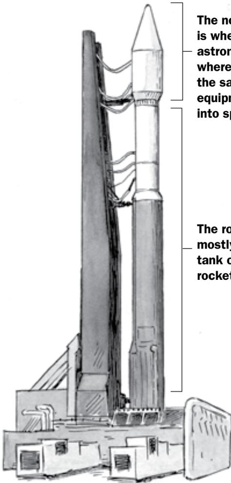
The nosecone is where the astronauts sit or where NASA stows the satellites or equipment it sends into space.
