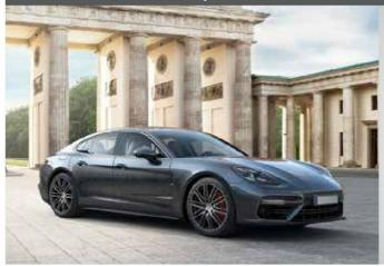
Porsche redesigned the Panamera completely for 2017; the hybrid version will hit the U.S. in summer 2017 as a 2018 model. It will have a 2.9-liter twin-turbo V6 that puts out 330 horsepower, a 136-hp electric motor, a 14.1-kWh lithium-ion battery, and an 8-speed automatic transmission. Total power output will be 462 hp and 516 lb-ft of torque. The claimed 0–60 mph time is 4.4 seconds, with a 31-mile electric-only range. AWD is standard.
