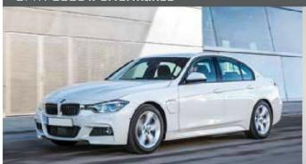
BMW's 3 Series plug-in, the 330e, features a 180-hp, 2.0-liter twin-turbo 4-cylinder engine, an 87-hp electric motor, a 7.6-kW lithium-ion battery pack, and an 8-speed automatic transmission with paddle shifters. Total horsepower is 248. The automaker claims a 0-60 time of 5.9 seconds and an all-electric range of 22 miles. EPA-estimated combined fuel economy is 30 mpg and 73 MPGe.
