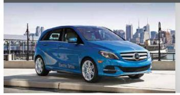
Mercedes-Benz's B250e EV is a compact but roomy five-person hatchback. Its powertrain combines a 177-hp electric motor with a 28-kWh lithium-ion battery housed under the vehicle's floor. The B250e's range is low for EVs these days, estimated at just 87 miles; a two-hour recharge is good for another 60 miles. The EPA-estimated MPGe is 84 in combined city/highway driving. The B250e is available in all 50 states, although most are sold in California.
