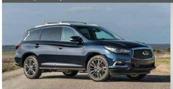
Full-size hybrid SUVs are few and far between. An exception is the Infiniti QX60 Hybrid, which has a 2.5-liter supercharged 4-cylinder engine, a 20-hp electric motor (good for 250 hp total), and is equipped with a CVT. The Q60 Hybrid is available with FWD or AWD. EPA fuel-economy estimates for both the FWD and AWD versions are 25 city/27 highway/26 in combined driving.
