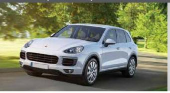
The Cayenne S E-Hybrid's drivetrain combines a supercharged 333-hp V6 and a 95-hp electric motor to produce 416 hp; they're mated to an 8-speed automatic transmission. The all-electric range is about 15 miles, and the EPA-estimated combined fuel-economy numbers are 47 MPGe on electric power and 22 mpg as a hybrid.
