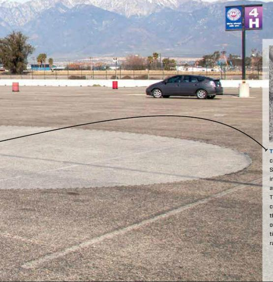
TURNING CIRCLE. A vehicle's turning circle is measured at the Auto Club Speedway. The right and left turning radiuses are measured, and the average becomes the turning circle. The vehicle with the largest circle receives a score of O, and the one with the smallest circle receives a 10. All other vehicles are then scored relative to the minimum and maximum radiuses.
