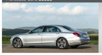
The S Class is Mercedes' flagship; its S550e plug-in hybrid's drivetrain consists of a 3.0-liter 329-hp twin-turbo V6 engine, a 114-hp electric motor (442 hp total), a 7-speed automatic transmission, and a water-cooled 8.7-kWh battery pack. The S550e can run solely on electricity for up to 12 miles. Charging on 240 volts takes under three hours; on 120 volts, about seven. Fuel-economy numbers are 26 mpg combined in hybrid mode and 58 MPGe running on electricity.
