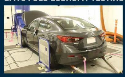
he EPA determines its fuel-economy ratings by performing tests on a dynamometer, a sophisticated treadmill-like device for cars that reproduces the load a vehicle experiences on the road under a variety of driving conditions. Its testing procedures are developed by recording motorists' driving patterns and creating "drive cycles" that represent those patterns.
