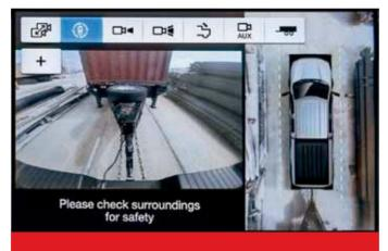
The latest cameras provide drivers with views all around a vehicle, as with the Ford F-150's MULTIPLE-CAMERA DISPLAY.
