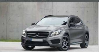
The GLA is Mercedes' compact luxury crossover. The most fuel-efficient version is equipped with a turbocharged 2.0-liter 4-cylinder engine that produces 208 hp and 258 lb-ft of torque and is matched with a 7-speed automatic transmission. An engine stop-start feature is standard. EPA-estimated fuel economy is 24 city/33 highway/27 combined for the FWD version; the AWD version achieves 23/31/26. The GLA250 is relatively quick for its class, with a 0-60 mph time of about 7 seconds.
