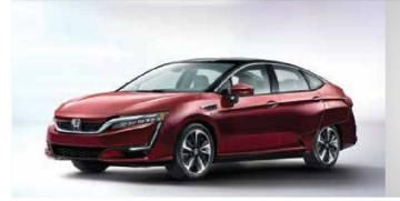
The Honda Clarity Fuel Cell's powertrain fits entirely under the car's hood, allowing for five-passenger seating. Its driving range is an EPA-estimated 366 miles, along with 68 MPGe combined. Honda began delivering the Clarity Fuel Cell to select California dealers in mid-December 2016. The lease price is \$369 per month for 36 months, with \$2,868 due at signing; \$15,000 worth of hydrogen fuel is included. Honda is planning to produce hybrid and EV versions of the Clarity in the near future.
