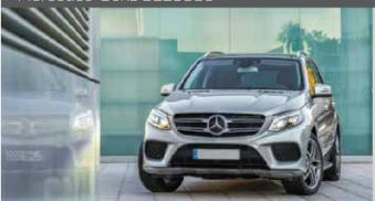
The GLE550e is powered by a 3.0-liter twin-turbo V6, good for 329 hp, and a 114-hp electric motor (436 hp total); a 7-speed automatic transmission; and an 8.8-kWh lithium-ion battery pack. M-B's AWD system, 4MATIC, is standard. All-electric driving is estimated at about 12 miles, and the recharging time is expected to be two hours on 240 volts or four to five hours on 120 volts. Fuel-economy figures are 21 mpg combined when running as a hybrid and 43 MPGe in all-electric mode.
