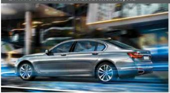
BMW's plug-in hybrid variants, the flagship 7 Series sedan (shown) and its X5 SUV, share drivetrain components: a twinturbo 2.0-liter 4-cylinder engine that makes 245 hp and a 95-hp electric motor, good for 320 hp combined; a 9.9-kWh lithiumion battery; AWD; and an 8-speed automatic transmission. The EPA-estimated combined fuel economy is 27 mpg and 64 MPGe for the 740e and 24 mpg and 56 MPGe for the X5. The EPA estimates the electric-only range at 14 miles for each.
