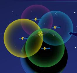
GPS receivers (your smartphone included) work by figuring out how far away they are from a number of satellites. They are programmed to know where the GPS satellites are at any given time.
