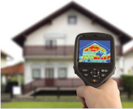
A home energy professional may conduct a thermographic inspection to find air leaks in the home.
